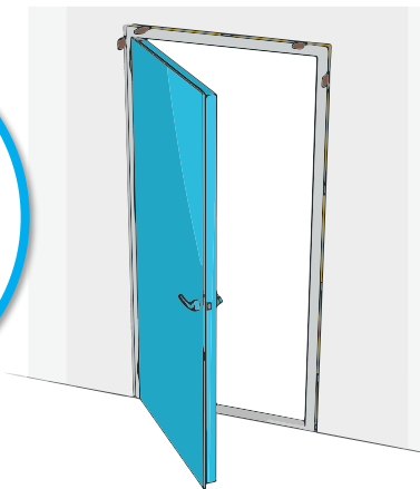
4 Fit doorleaf on hinges and check door clearance.
